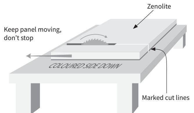
Figure 8: Cutting with Table saw
