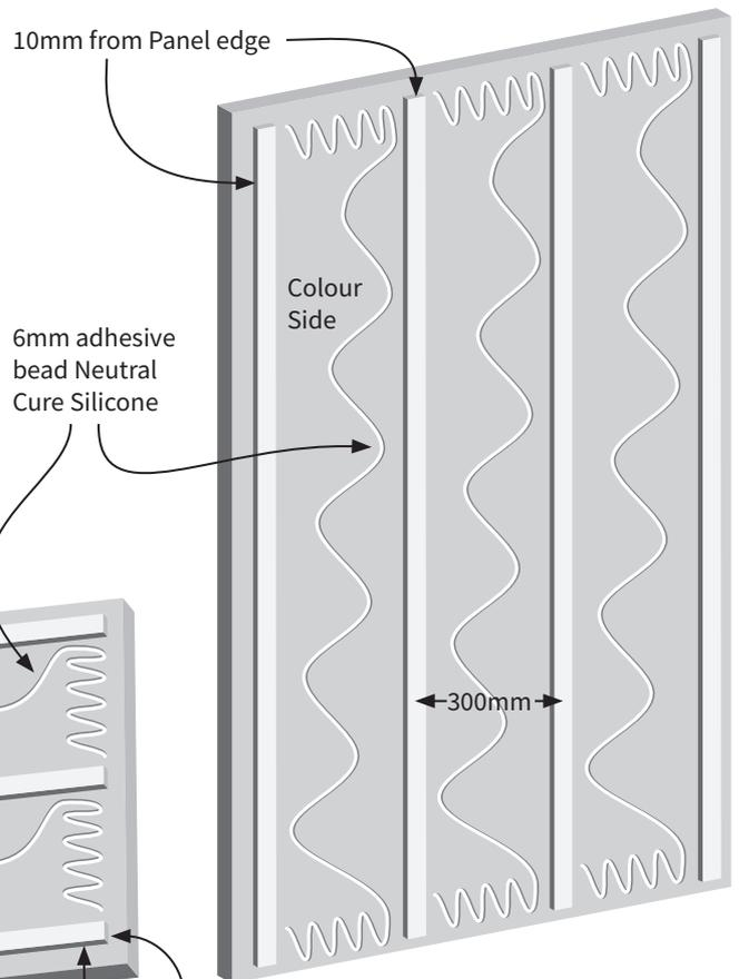
Figure 21: Apply Tape and Neutral Cure Silicone - Vertical Panel
