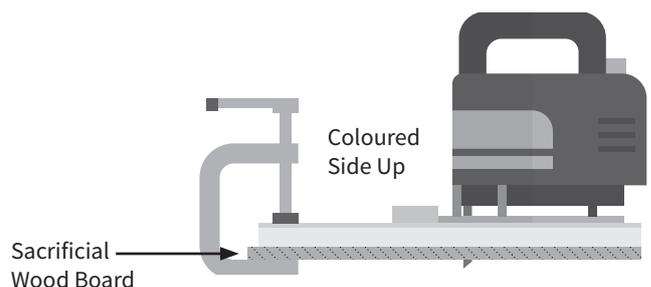
Figure 15: Cutting with Jigsaw Colour Side Up
