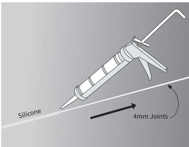
Figure 22: Sealing Joints
